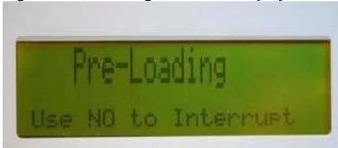
NOTE: During Pre-Loading the actuator always returns to the start position of the last infusion programmed.
