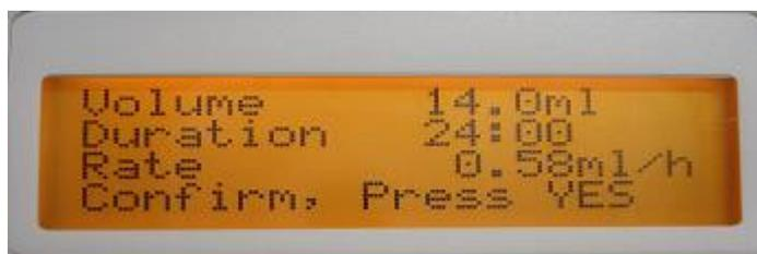
ii. The McKinley T34 Syringe Pump calculates and displays the deliverable volume, the duration of the infusion (24 hours) and the rate of the infusion (ml per hour). Press the “YES” key to confirm the details. The display screen prompts “Start Infusion?”
